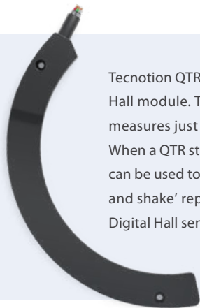
Digital Hall module mounted* on QTR-A 65 series
