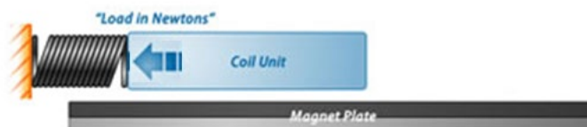
Picture 5 - In this example an external force is applied through a spring, which only exerts a force when it comes in contact with the coil unit. This means that only profiles dealing with that particular stage of the movement cycle should have a value for 'Load'.
